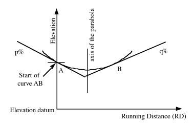
A practical formula for a general parabola for a vertical curve is therefore
