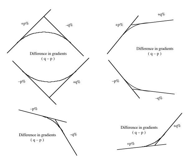
The convention with vertical curves is that they are drawn and computed going from left to right. If the grade is rising from left to right, the gradient is positive. If it is going down from left to right, the gradient is negative. The above diagram shows the signs that the various gradients would take in the circumstances.
