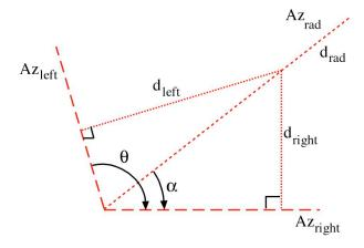
The angle  $\theta$  is the difference between the two known azimuths,  $Az_{left}$  and  $Az_{right}$ . The offset from the right traverse line to the object is  $d_{right}$ , while the offset from the left traverse line to the object is  $d_{left}$ . Because the offsets are measured at right angles to the traverse lines, their azimuths are also known.
