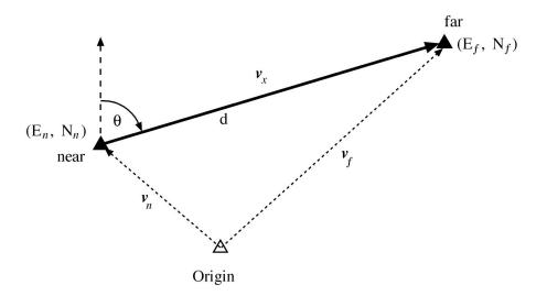
2. Using vectors, as shown in the figure above, the co-ordinates of each point are entered as the components of a pair of 2-D vectors. In the HP-35s, 2-D vectors are best handled as complex numbers, so that the co-ordinates are stored as the two vectors from the origin,  $\mathbf{v}_f$  and  $\mathbf{v}_n$ , as follows:
