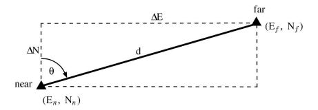
1. Using co-ordinates alone, as in the figure above the differences between the easting coordinates of the points ( $\Delta E$ ) and difference between the northing co-ordinates of the two points ( $\Delta N$ ) are obtained. The point from which the azimuth is desired to come is termed the 'near' point, while the point to which the azimuth points is termed the 'far' point. So:
