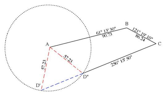
Using the above situation as an example, line AC is the resultant vector from the vector addition of the sides AB and AC. This vector is 90° 25' 53" for 153.204. The triangle to be solved forms as below. Note that the AD'D" triangle is isosceles.
