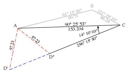
Using the sine rule to solve for the angle at D, the following occurs:
