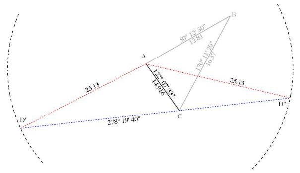
The azimuth of the line AD' is therefore  $98^{\circ} 19' 40'' - 13^{\circ} 51' 27'' = 84^{\circ} 28' 13''$  and using the sine rule gives 38.047 for the length of CD'.
