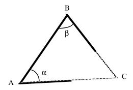
Any plane co-ordinates may be used, using any units of distance measurement. Angles are expected in degrees, minutes and seconds, using HP notation. The solution assumes that plane surveying conditions apply, but this will usually be the case with this type of work and the precision expected will be such that any small differences caused by geodetic considerations will be within the range of likely random errors.
