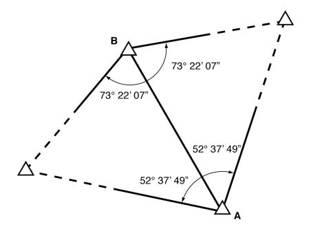
The first solution is to the 'left' of the line from A to B, while the alternative solution is to the 'right' of the line from A to B. You should look at both solutions and check which of the solutions is the one you want.
